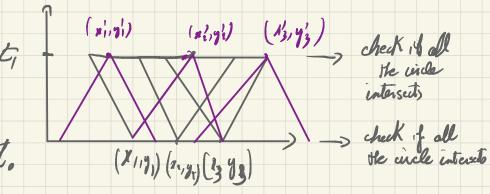
\_ So, our problem now, quien n circles in 1R2 how con me check if all intersects or not pick two circles  $C_i = (P_i, r_i) & C_i = (P_i, r_i)$ where Bk is the center & Tk is the radius, K = 1,39. C; naterscito C;  $\iff$   $d(P_i,P_j) \iff P_i+P_j$ . So, the olyonithm mill pick any two circles. & check of they intersect, of they don't it can return " no pomble meeting" - otherwise, it will compute the intersection points + the curves that cornect them. (there one 2 intersection points).
